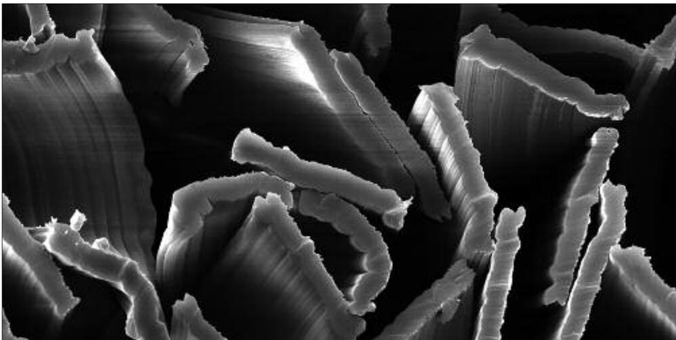
Figure 1: Viloft short cut fibers have high stiffness on the narrow side and low stiffness on the long side.
