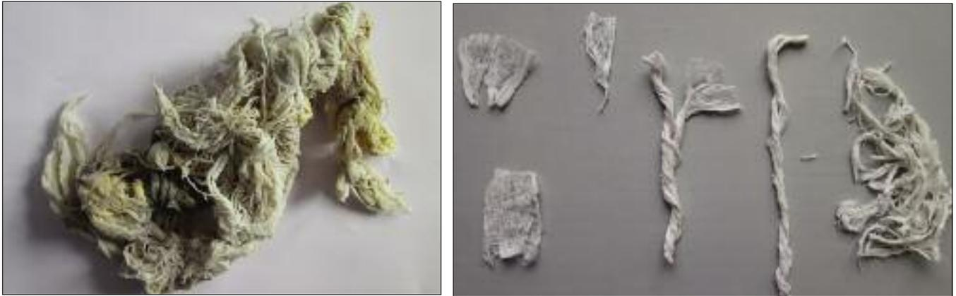
Figure 2: Analysis of a real blockage found in one of the pumps of AZV Saal: the cause is undispersed wet wipes (e.g. baby wipes). All samples contained polyester and long viscose fibers and were manufactured in typical spunlace processes (for high strength).
